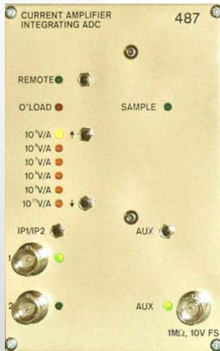
The 487 is used as the main amplifier in DC systems employing current source detectors such as photomultipliers and photodiodes (eg. Si, Ge, InGaAs) which, at low frequencies, give their best performance when connected to a virtual ground. The typical spectral range over which these detectors, and therefore this amplifier, are used is 180nm to 1700nm.
