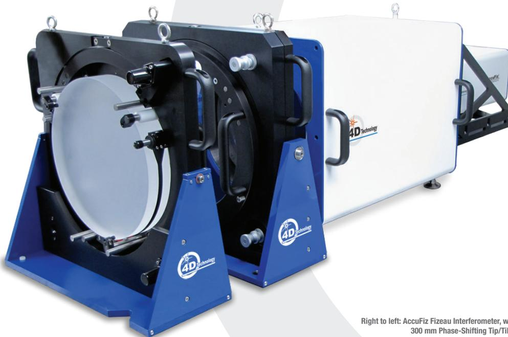
Right to left: AccuFiz Fizeau Interferometer, with 100-300 mm Aperture Converter, 300 mm Phase-Shifting Tip/Tilt Mount and 300 mm Tip/Tilt Mount.
