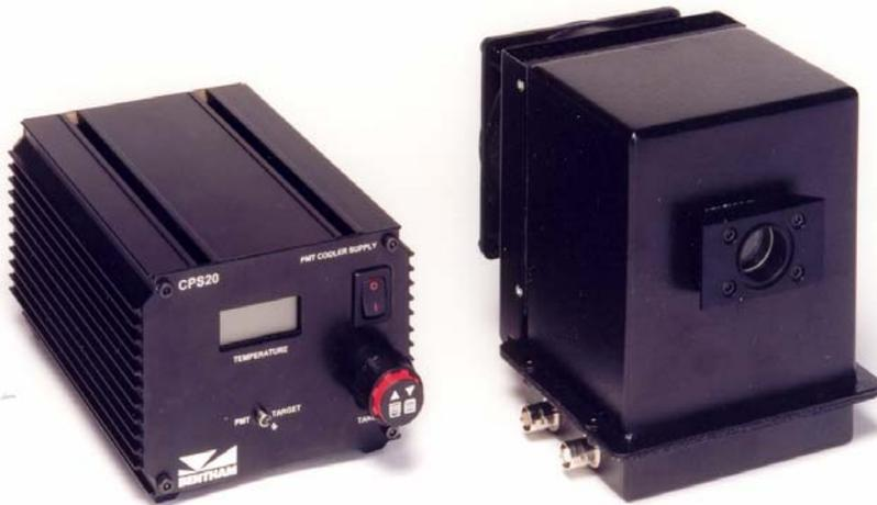
The DH-00-Te cooled housing accepts all 28mm (1 1/8 inch) diameter side-window photomultiplier tubes. It has been designed to be integrated easily and unobtrusively into light measurement systems where dark current or temperature dependent gain variations\* need to be minimised. Minimum internal temperature is -25°C and stability better than  $\pm 0.1^\circ\text{C}$ . For a multi-alkali pmt, dark current is typically reduced by a factor of 100\*\*.
