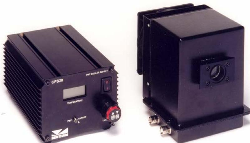
The DH-00-Te cooled housing accepts all 28mm (1 1/8 inch) diameter side-window photomultiplier tubes. It has been designed to be integrated easily and unobtrusively into light measurement systems where dark current or temperature dependent gain variations\* need to be minimised. Minimum internal temperature is  $-25^{\circ}\text{C}$  and stability better than  $\pm 0.1^{\circ}\text{C}$ . For a multi-alkali pmt, dark current is typically reduced by a factor of 100\*\*.
