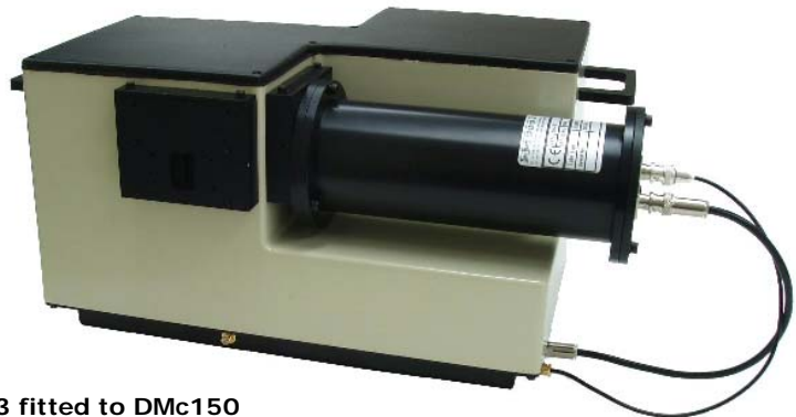
DH-3 fitted to DMC150 monochromator
