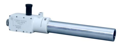
The Model D-275 Autocollimating Alignment Telescope can be focused from 16 inch (406.4 mm) to infinity, to align any number of points along its optical axis. Due to the fact that the mechanical axis of the tube and the optical axis of the instrument are parallel within 3 arc seconds, the instrument is easily adaptable to jigs and setups using a dial indicator.
