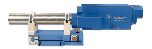
The Model D-275-AAT Automatic Autocollimating Alignment Telescope focuses from 16 inches (40cm) to infinity, to align and measure the location and angular orientation of any number of targets along its optical axis. Since the mechanical axis of the tube and the optical axis of the instrument are parallel within 3 arc seconds, the instrument is easily adaptable to mounts, jigs, stages, and various setups and setups using a dial indicator.
