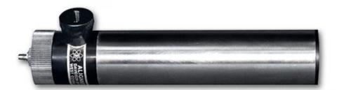
This small precision Alignment Telescope is rugged, versatile and easy to use. It will align points along its optical axis to better than  $\pm.010$  inch (0.25 mm) up to 35 feet (10 m) away. Mechanical fixturing is made easy because the barrel is parallel to the optical axis. With the added feature of an autocollimator, reflective surfaces can be aligned perpendicular to the D-271.
