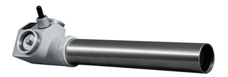
The Model D-660 straight through Two Axis Autocollimator is capable of repeating angular measurements to  $\pm 0.1$  arc second. The two micrometer readout dials are independent of each other and have separate eyepieces for reading their scales. The standard 2.249 inch (57 mm) diameter barrel makes interchanging this instrument with other mounts or using V-blocks easy. With the Model D-165 High Intensity Light Source, Fiber Light Guide and Adaptor the Model D-660 can also measure uncoated parts.
