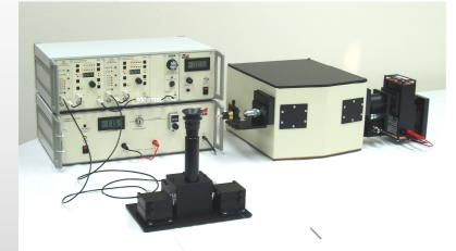
The Bentham Fibre Spectral Loss System is modular in nature and consists of chopped light source, monochromator, launch optics, detector and lock-in amplifier. The whole system is controlled by a PC which also calculates loss in dB/km as a function of wavelength.
