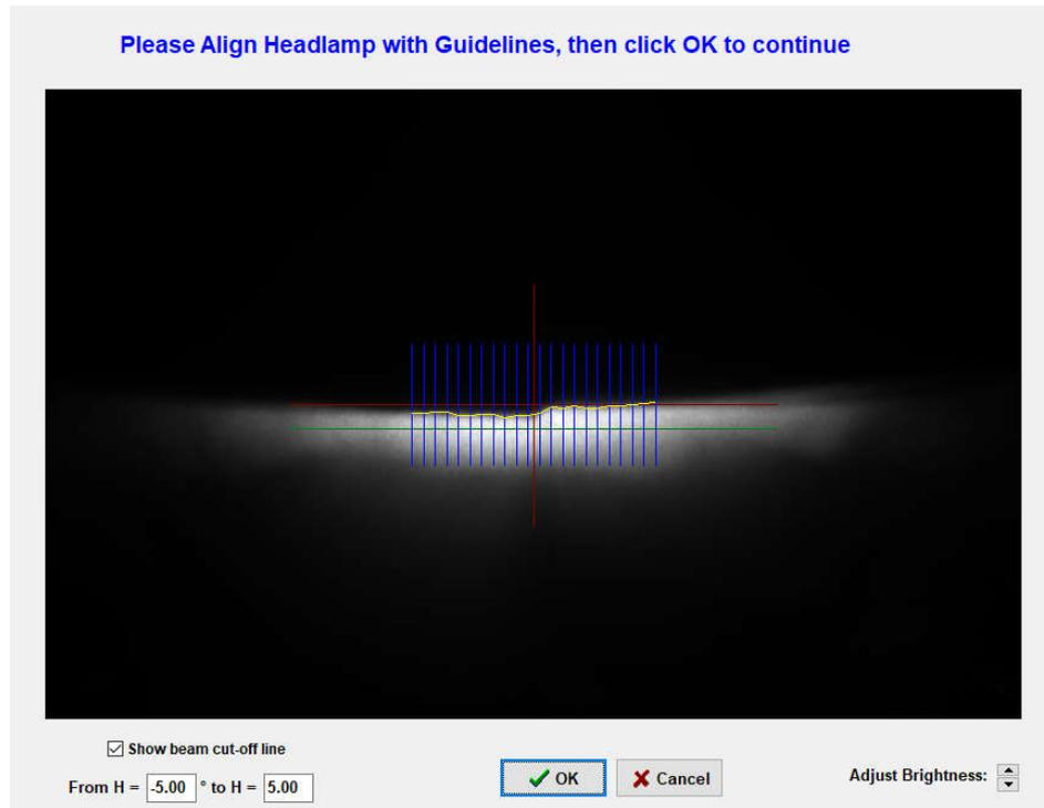
**Figure 13: Align low beam**
