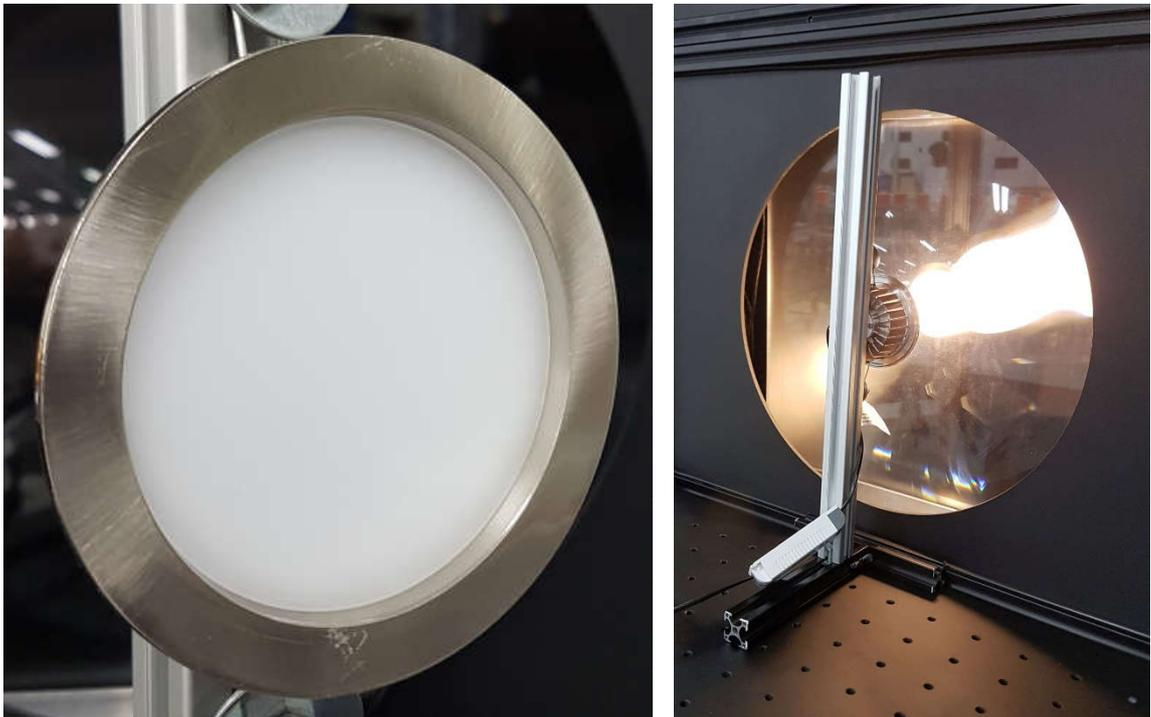
**Figure 37: Flat field calibration source**
