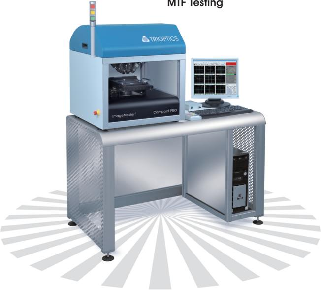
The ImageMaster® Compact PRO is a production MTF tester for qualifying mobile phone and other miniature lenses measuring objective lenses with an effective focal length between 1 and 12 mm. The instrument is opti-
