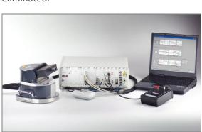
The interferometer has a resolution of 1 nm at a maximum range of 15 m. The influence of the environmental conditions is compensated by implemented temperature, pressure and humidity sensors. The laser tube is located in the external control box and guided to the Laser-TRACER by a glass fibre. Therefore the thermal load is greatly reduced and a compact design can be provided. The LaserTRACER can be handled by a single operator and is applicable to machines of all working volumes.
