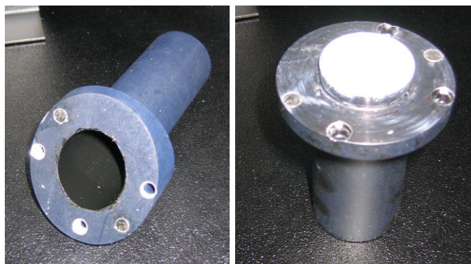
Figure 5: Gloss Trap and Diffuse Reflecting Plug for Measurement of Specular and Diffuse Reflectance
