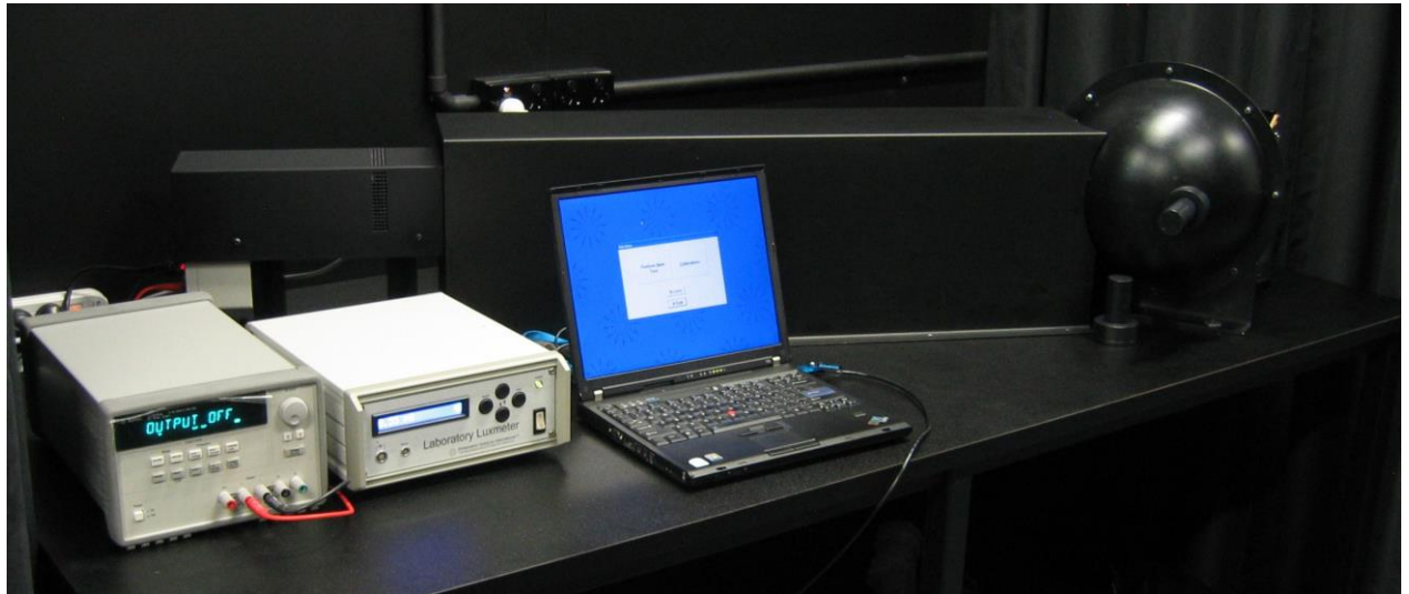
Figure 2: Mirror Reflectometer Set-up
