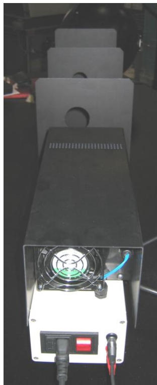
Figure 3: Back of Collimated Source and Baffles Leading to Sphere
