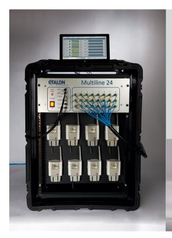
▷ The absolute Multiline system in a rugged box for mobile application (with an 8 channel wireless temperature system)
