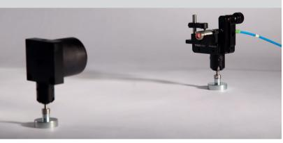
▷ A single measurement channel consists of a miniature optical element connected to a single fibre and a reflector
