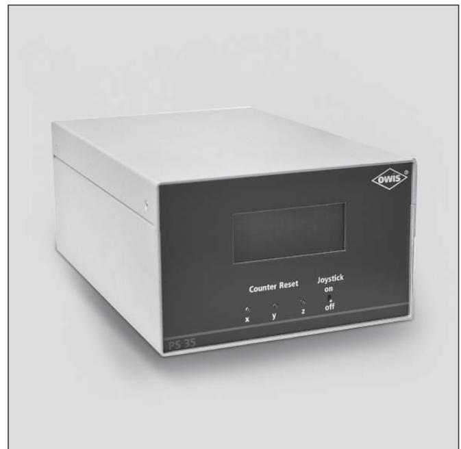
The PS 35 as an universal position control unit in a table top with LCD controls up to three axes of 2 phase step motors or DC servo motors (brush). Different combinations of both motor types are possible. The display shows the status of each axis and its position with measuring unit. Further, for each axis a reset button is provided.
