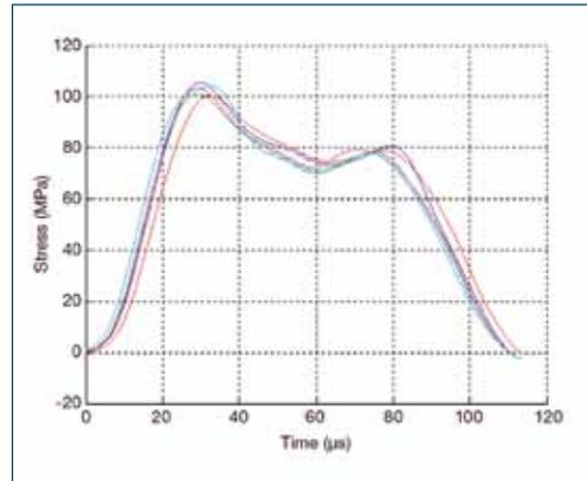
Image 3: typical double-pulse shape with the seismic mass
