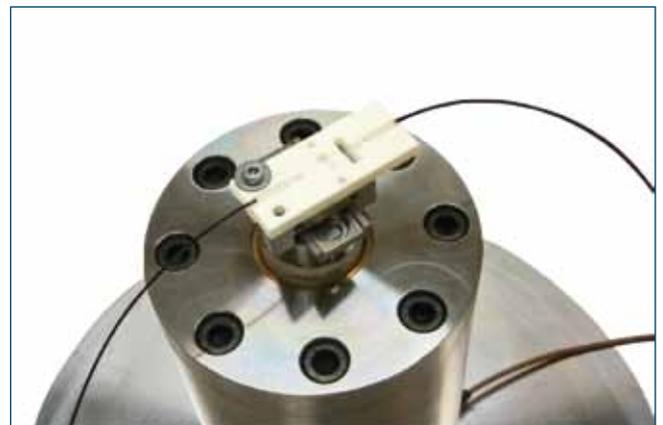
Image 6: Geoshaker with seismic mass
