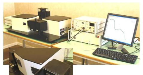
The SSUV300 performs the accurate measurement of UV transmittance through thin film sunscreen samples in strict accordance with the COLIPA guideline "Method for the In Vitro Determination of UVA Protection Provided by Sunscreen Products".
