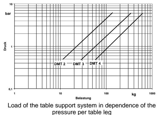
The advantage of this bearing is the low-frequency tuning of the system which results in an effective isolation against floor concussion. The vertical characteristic frequency of this support is lower than 0,85 Hz. Assuming floor concussions with resonance above 8 Hz this corresponds to a degree of insulation of more than 90%.The lateral characteristic of the bearing system is dependent from the set up.
