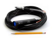
The miniLDV probe, the size of a small flashlight, is self contained and permanently aligned; no calibration required by the user. The probe contains a laser, miniature beam shaping optics, receiving and detection optics.
