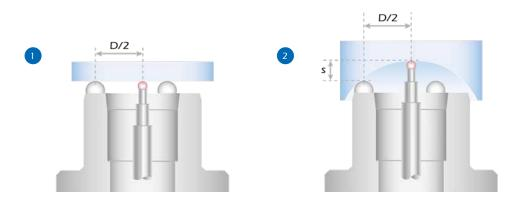
Determination of the reference position using a precision optical flat.
