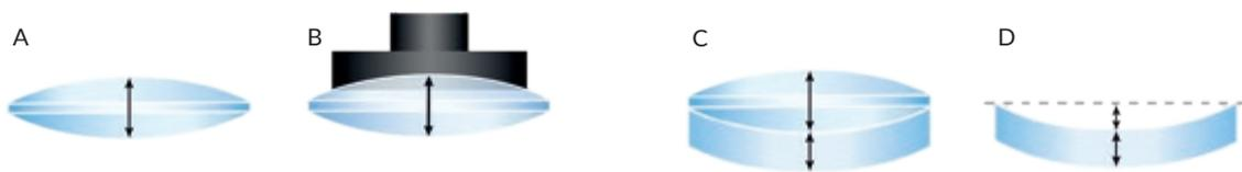
OptiSurf® LTM enables the measurement of single lenses without (A) and with (B) arbors, doublets (C) and the sag value (D).
