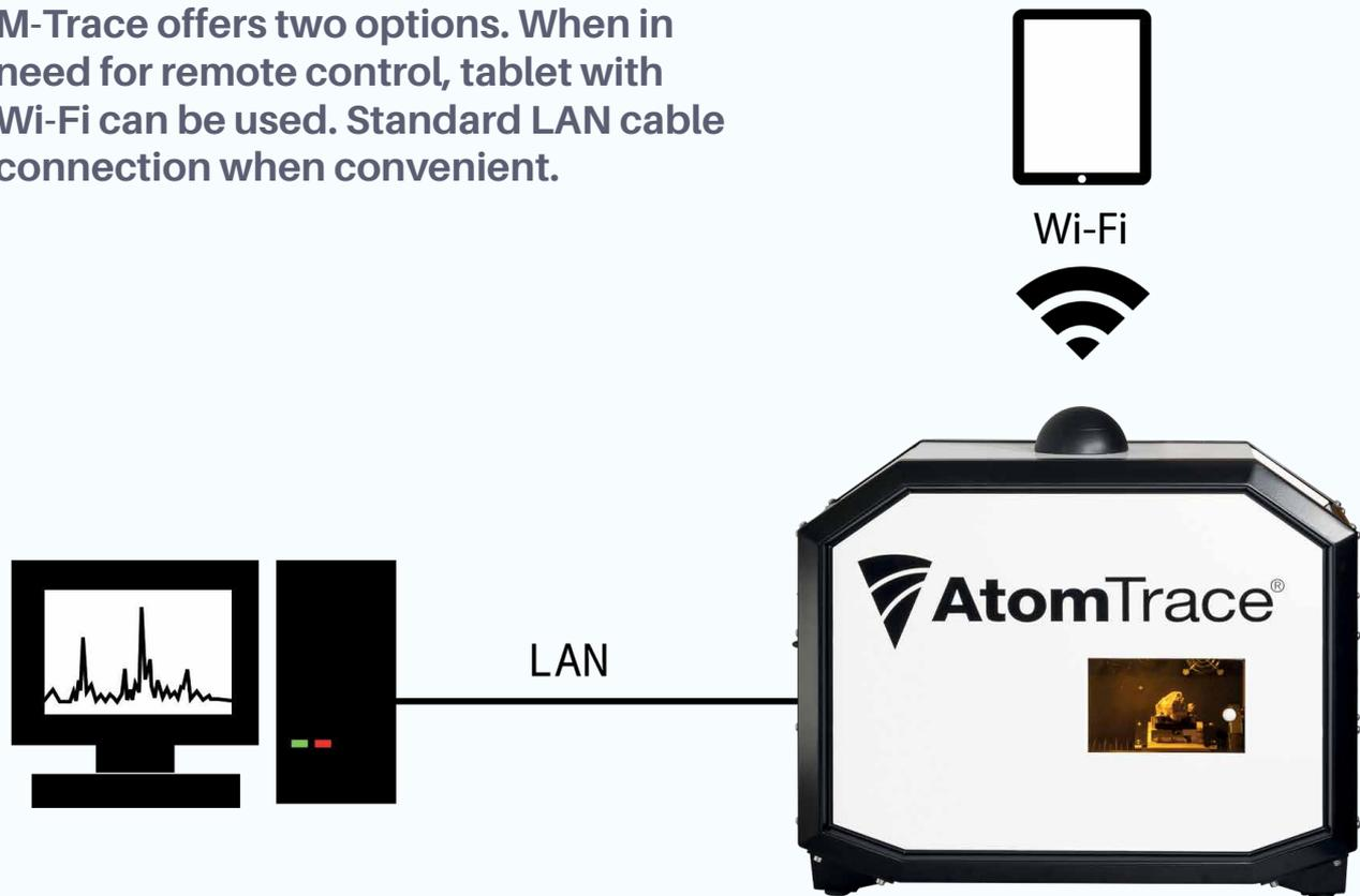
The client-server architecture detaches control and allows remote manipulation with the device via network communication channels Wi-Fi 2.4 GHz, 5.0 GHz, GSM, 3G and LTE. Measured LIBS data are along with initial outputs from analysis saved in real time to local data storage in the device. In the sense of Industry 4.0, the measured LIBS data along with the outputs of the analysis could be exported to remote data storage units on the servers or cloud.
