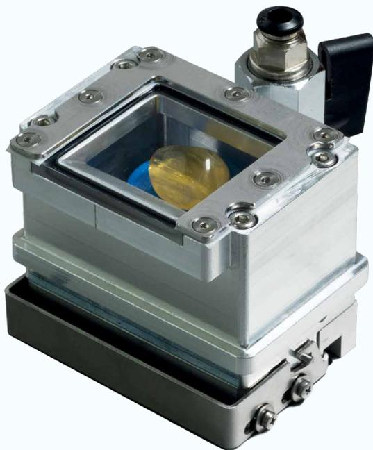
Vacuum helps to isolate signal of elements: carbon, oxygen, nitrogen, hydrogen from the sample. Since ambient air contains these elements, signal from the sample measured in ambient air could be affected.
