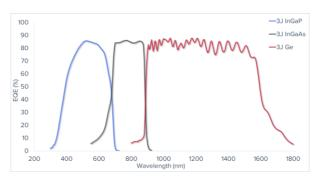
External quantum efficiency of InGaP, InGaAs and Ge three junction solar cell
