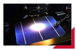
In poorer quality material, where the crystal structure is defective, there are traps and defects to which generated carriers are lost, leading to incorrectly reported spectral response.
