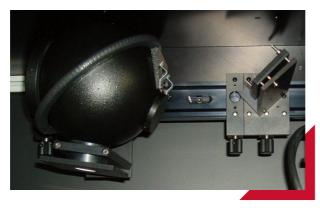
In addition to providing a manner of determining device IQE (below), these measurements also permit the characterisation of anti–reflection coatings and the transmission of thin film layers.
