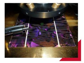
Care should be taken to ensure the probe beam is not shaded by electrical connections, or that the shading is taken into account by correcting the resulting response.
