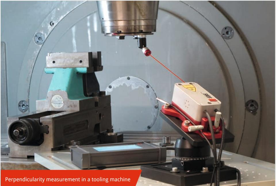
Perpendicularity measurement in a tooling machine
