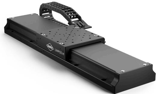
The LINPOS M combines a powerful direct drive with a fine resolution incremental linear measuring system, allowing high dynamics at highest precision. The ironless linear motor enables fast movement with constant speed up to 950 mm/s and the smooth rastering in small equidistant steps equally.
