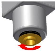
**2. Screw the flex-Adapter into the microscope.**
