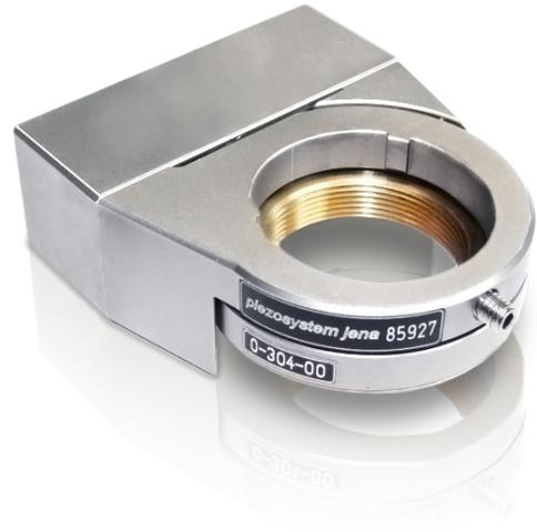
The objective lens positioning system MIPOS 100 was developed for finely adjusting objectives / lenses. The maximum motion is 100  $\mu\text{m}$ . The resolution of MIPOS 100 is very high and, in practice, only limited by the voltage noise of the power supply.
