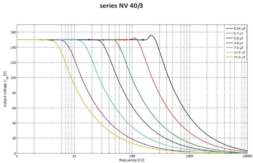
The diagram shows the typical frequency of the NV 40/3 series which can be reached as a function of the capacitance of the piezoelectric actuator and the driving voltage by an output current of 40mA.
