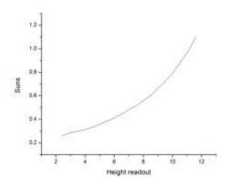
Typical attenuation behavior of the 11002 SunLite $^{\text{TM}}$  Solar Simulator using the model 15279 option.
