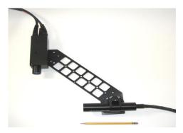
The 3D miniLDV probe is extremely compact, self contained, and permanently attached to a structure; no calibration or alignment by the user is required. The probe contains three high power lasers, miniature beam shaping optics, and detection optics.
