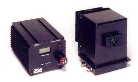
The DH-00-Te cooled housing accepts all 28mm (1½ inch) diameter side-window photomultiplier tubes. It has been designed to be integrated easily and unobtrusively into light measurement systems where dark current or temperature dependent gain variations\* need to be minimised. Minimum internal temperature is  $-25^{\circ}$ C and stability better than  $\pm$  0.1°C. For a multi-alkali pmt, dark current is typically reduced by a factor of  $100^{**}$ .
