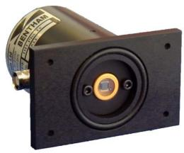
The DH-PbS-Te and DH-PbSe-Te are large area  $(3 \times 3mm)$  thermo-electrically cooled detectors. They are particularly suitable for accurate spectroradiometry and general spectrometry applications over the  $1\mu m$  to  $5\mu m$  range.
