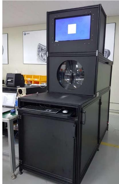
**Figure 2: The ICP-1.0 imaging photometer**
