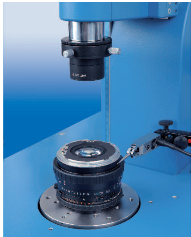
Measuring the lens barrel with the lever gauge
