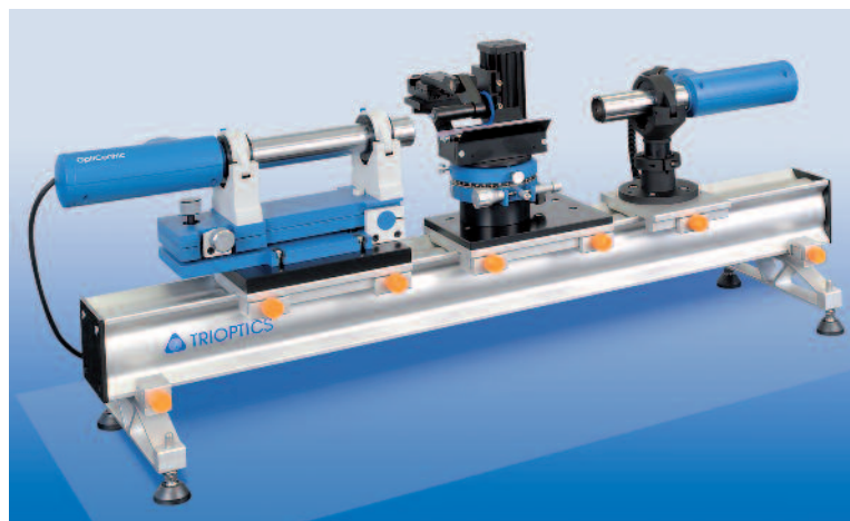
Customer specific instrument for the measurement of laser rod end surfaces
