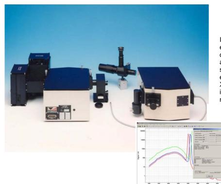
In order to fully characterise both excitation and emission spectra of phosphors, Bentham supplies a dual monochromator based system. Typically a dual excitation source comprising Xenon and quartz halogen lamps is fitted to the excitation monochromator and PMT, silicon and InGaAs detectors can be fitted to the emission monochromator, therefore both excitation and emission spectra can be measured from 200nm to beyond 1800nm.
