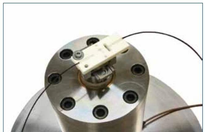
Image 6: Geoshaker with seismic mass
