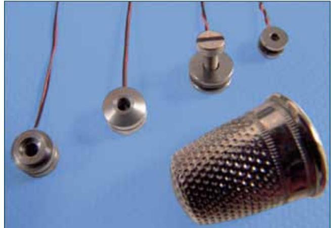
Image 7: different micro-shaker. size comparison with thimble
