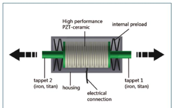
Image 1: Scheme of a symmetric acting shock generator working in axial direction
