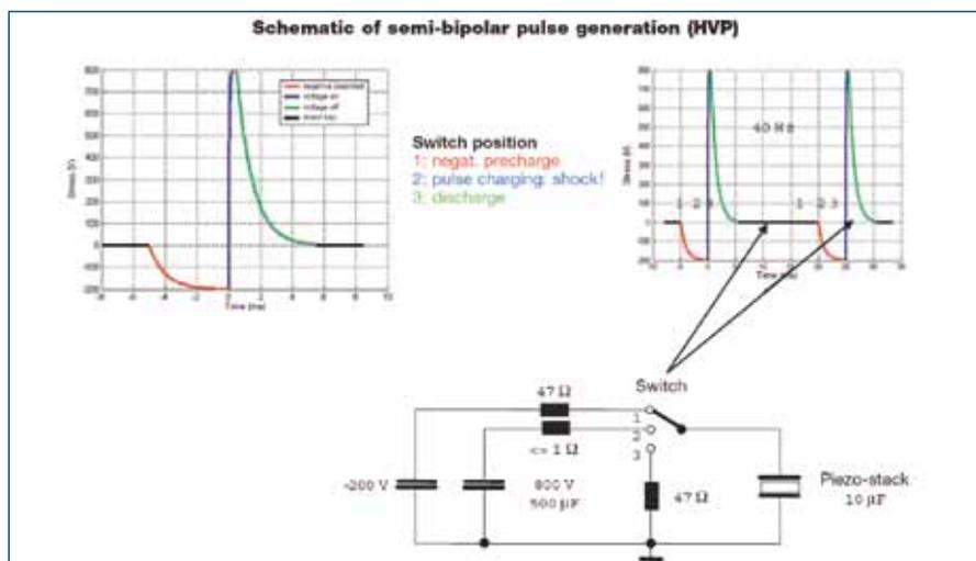
Image 4: schematic bipolar control of a power piezo actuator by a high-voltage-pulser (HVP)
