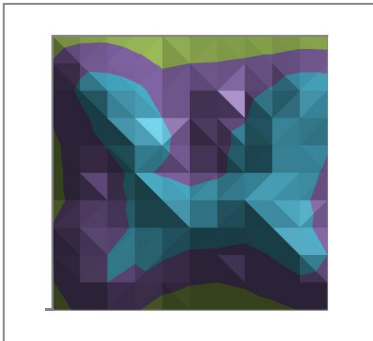
Non-uniformity map of an Abet Technologies model 11016 Solar Simulator, 110x110 mm, 3%.
