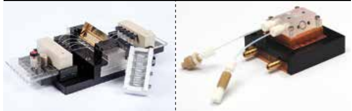
In situ SPR cell allowing kinetic SPR measurements
