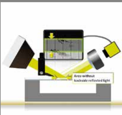
Knife edge illumination allows the investigation of thin transparent substrates
