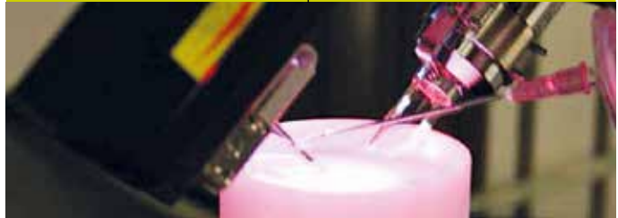
Light guide enables measurements at liquid/liquid interfaces and solid/liquid interfaces at variable angles between 40° and 72°
