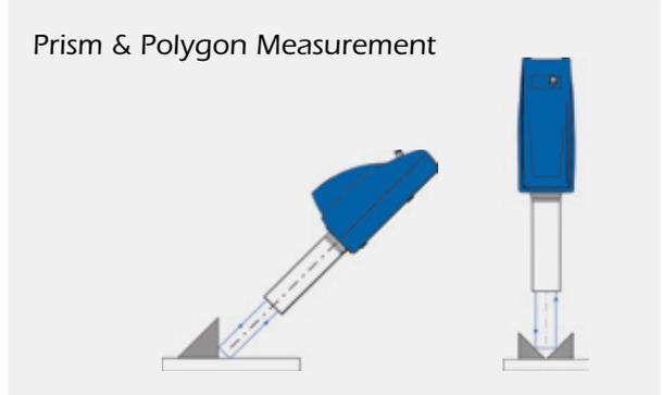
Alignment of Optical Components
