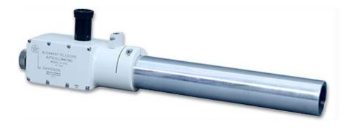
The Model D-275 Autocollimating Alignment Telescope can be focused from 16 inch (406.4 mm) to infinity, to align any number of points along its optical axis. Due to the fact that the mechanical axis of the tube and the optical axis of the instrument are parallel within 3 arc seconds, the instrument is easily adaptable to jigs and setups using a dial indicator.
