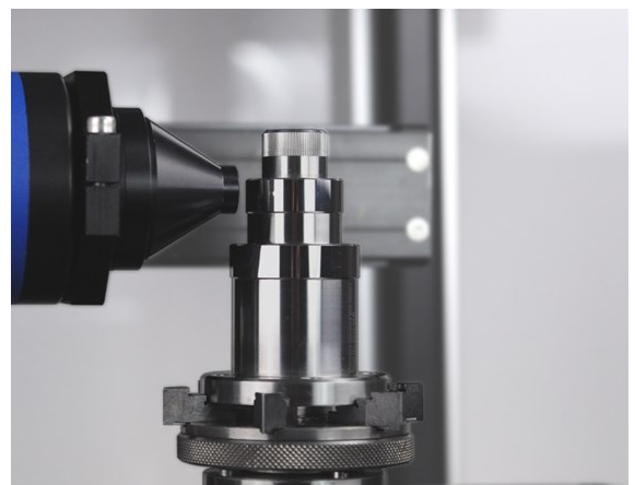
Measurement on a waviness standard WS 300/01
