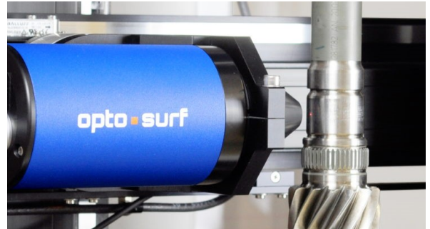
Automatic approach to a measuring position on a gear shaft.
