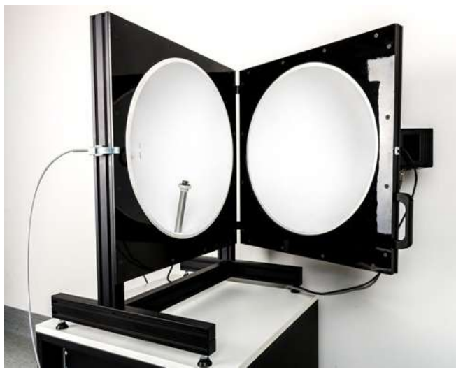
Fig. 3. GL Opti Sphere 500 integrating sphere with a universal lamp holder.
