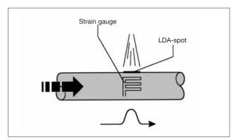
Figure 1: Schematic of a shock wave propagation within a solid bar, detected by strain gage and LDA measurements.
