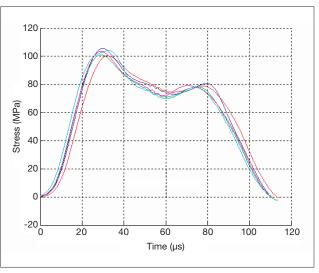
**Figure 11:** Mechanical stress/time profile time for a burst of shocks. Active stack length: 120 mm. Shockwave energy: 3.25 J. Take notice of the remarkable coincidence of the mechanical pulses.
