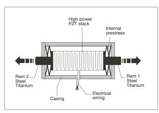
*Figure 4a:* Schematic of a symmetrical piezo-shock-generator.
