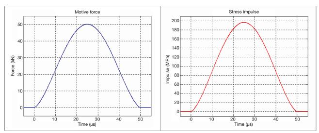
Figure 13: Force of contact as a function of time (left) and stress impulse as a function of time (right).
