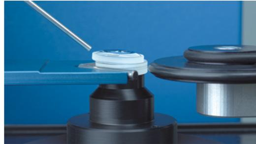
Lens alignment with the LensAlign 2D Air on a lens rotation device
