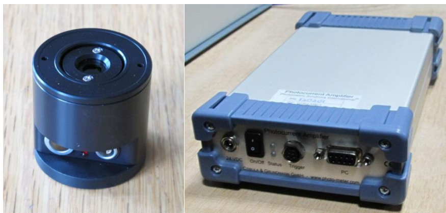
Figure 4: Photocell and Amplifier
