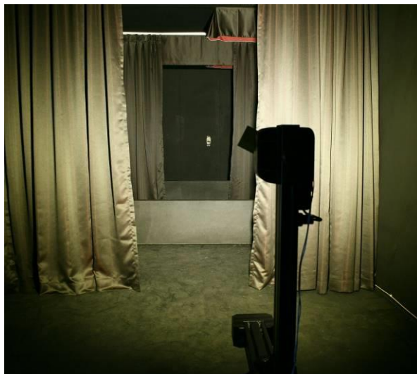
Figure 12: Curtains and wooden panels for baffling
