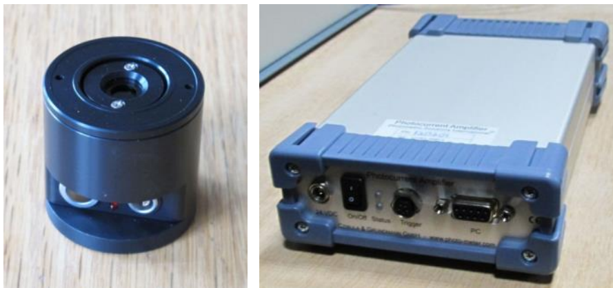
Figure 4: Photocell and Amplifier
