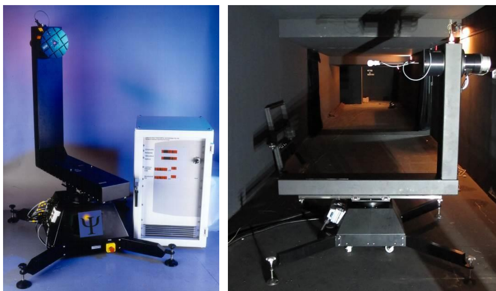
Figure 1: The LG-1.5: (Left) Shown with a 19" Cabinet and old PSI logo (Right) Shown in a dark room before stray light baffles are installed.
