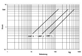
Load of the table support system in dependence of the pressure per table leg
