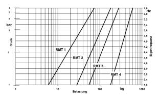
Vertical Characteristic frequencies of the Table Support System RMT in dependence of load per table leg.
