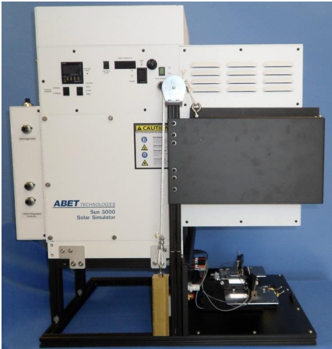
Abet Technologies' Model 15500 Stage with Model 15501 magnetic base and Model 15504 Dark enclosure in use with a Sun 3000 Solar Simulator
