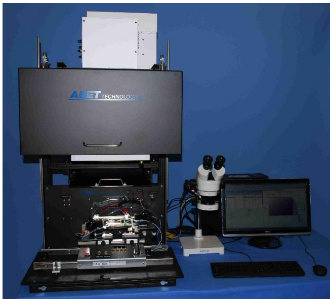
Abet Technologies' Model 15510 Stage with a large selection of its optional accessories in use with a Sun 3000 Solar Simulator
