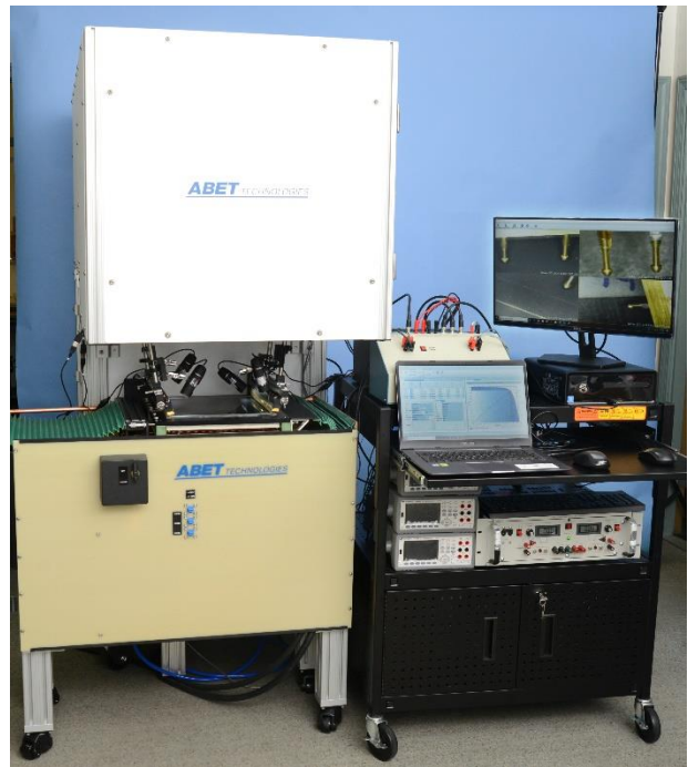
Model 15530SP 300x300 mm stage motorized chuck for CIGS mini-modules for automatic single cell and full mini-module IV metrology in use with a Sun 3000 Solar Simulator, a 15295 100V electronic load and four alignment microscopes. The simulator equipped with a filter wheel for Red and Blue and Attenuated measurements.
