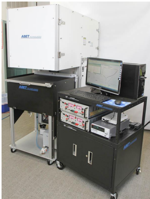
Model 15530 300x300 mm stage with dark enclosure closed generating a dark IV curve using 15295 Universal load.
