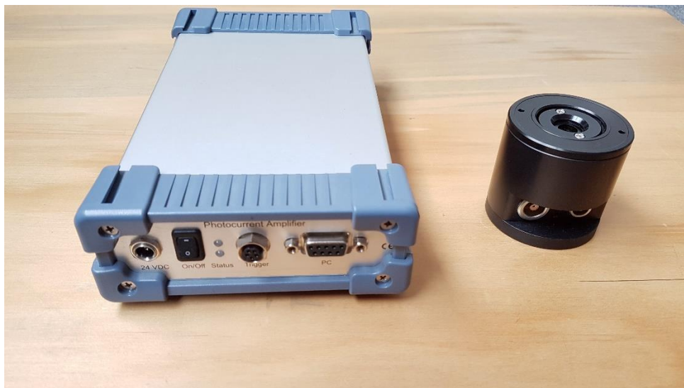
Figure 1: Photocell and amplifier
