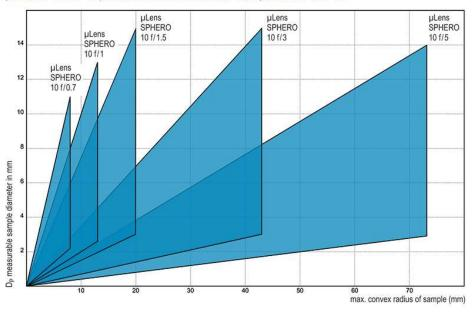
µLens SPHERO objectives for combination with µLens PLANO 50
