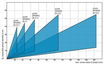
$\mu Lens$  SPHERO objectives for combination with  $\mu Lens$  PLANO 100 and 150 on request
